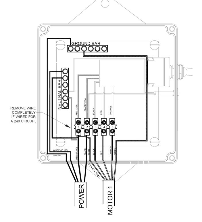
For clarity, the terminal connections have been numbered 1-5 from left to right in the figure above. The terminal connections are not labeled inside the Bonita unit.
