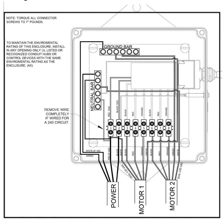
For clarity, the terminal connections have been numbered 1-8 from left to right in the figure above. The terminal connections are not labeled inside the Bonita unit.
