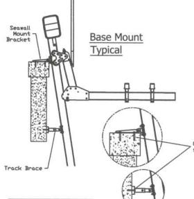
Concrete anchors, 5/8'\$ min stainless steel
