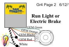
Attach the run light to the GEM Red & a neutral (120) even though the motor is wired for 240VAC.
