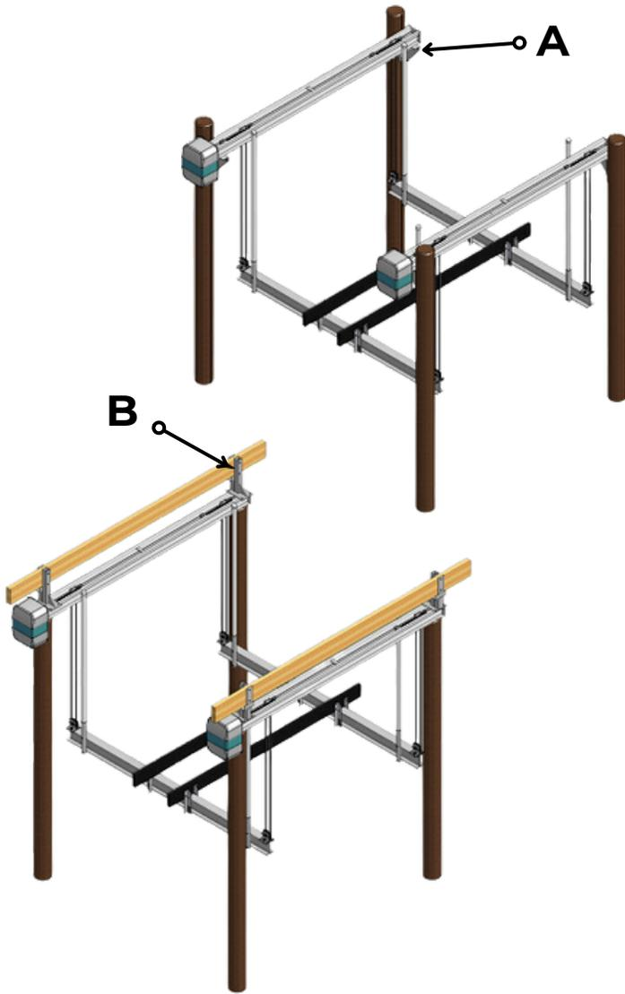
**A** Side mount brackets are used for mounting standard top beam lifts to piling when the top of piles are not accessible or other mounting means are not available.
